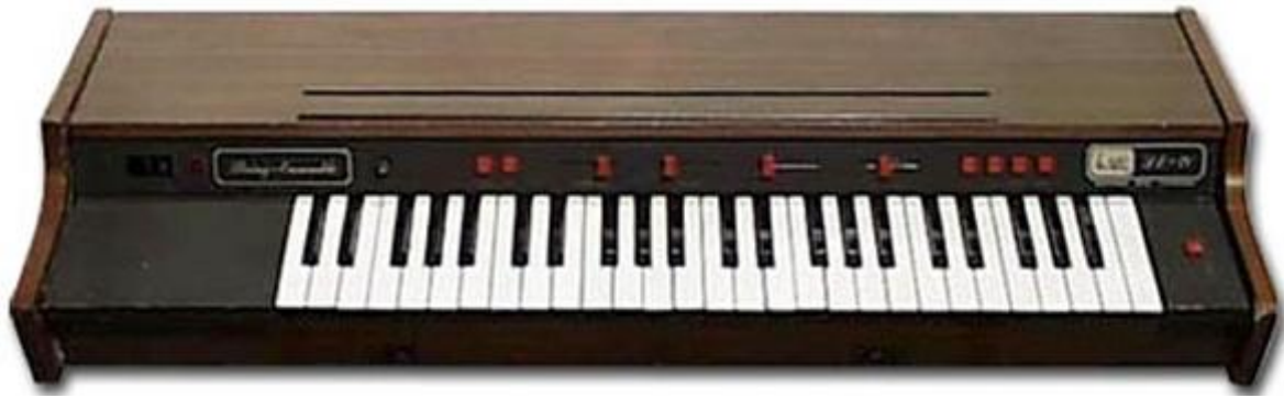
Figure 24 - The ARP "Solina" String Ensemble Synthesizer
