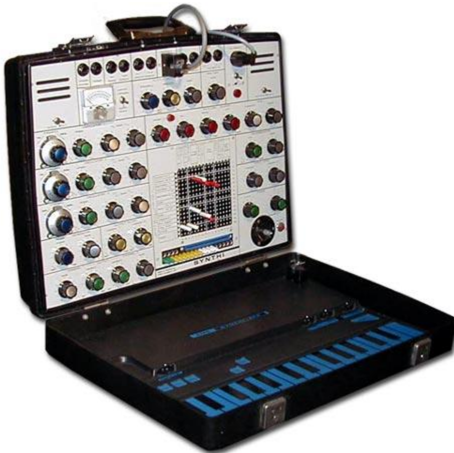
Figure 16 - EMS VCS3 Synthi AKS - Essentially, a Synthi A with a Keyboard & Sequencer compartment
