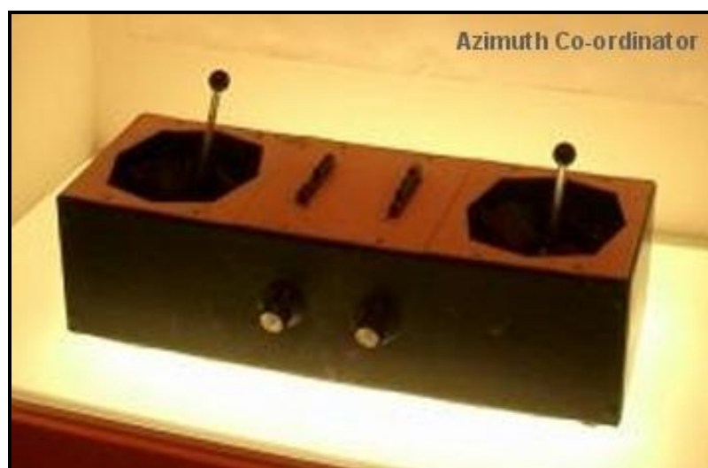
Figure 2 - Azimuth co-ordinator 'quadraphonic' pan system (from the Paris Interstellar Exhibition)
